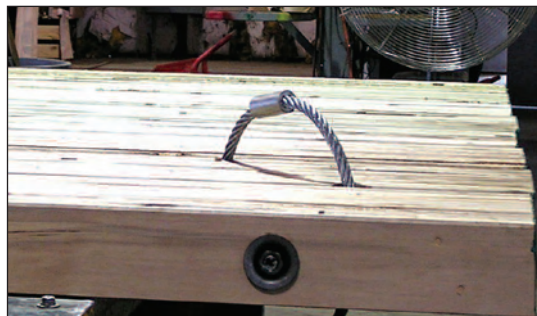
Then, steel dowl rods are inserted and bolted in place before loading onto trucks for shipment. ▶
