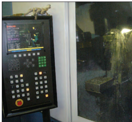
One of the newest additions to the Bibler plant is the computer-controlled saw sharpening system by Vollmer. This state-of-the-art machine can sharpen an average of 12 saws per hour with incredible precision.
