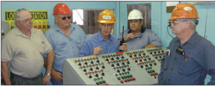
Koppers operates four 146-foot-long treating cylinders with a capacity of 800 nine-foot ties per charge for more than 1.5 million ties per year. Maxey (center) and Paul (right) explain how automation of each of the plant's treating cylinders maximizes efficiency.
