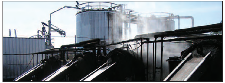
Koppers operates four 146-foot-long treating cylinders with a capacity of 800 nine-foot ties per charge for more than 1.5 million ties per year. Maxey (center) and Paul (right) explain how automation of each of the plant's treating cylinders maximizes efficiency.
