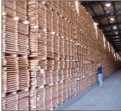
And what impressive drying/conditioning operations for hardwood lumber! The airflow through this warehouse pre-dryer alone pulls out up to 10,000 gallons of water per day. They can condition 2.5 million board feet in this location at one time.
