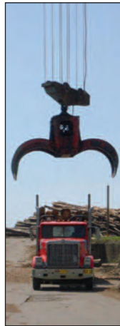
The log crane operator is in constant contact with every driver, and the crane can off-load up to 60,000 pounds in a single lift. Bibler off-loads up to 180 trucks a day.
