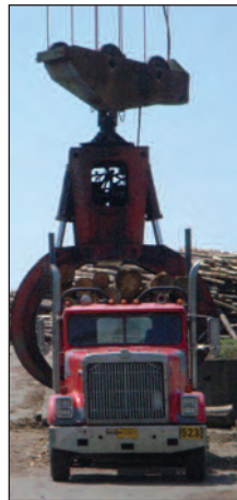
The log crane operator is in constant contact with every driver, and the crane can off-load up to 60,000 pounds in a single lift. Bibler off-loads up to 180 trucks a day.
