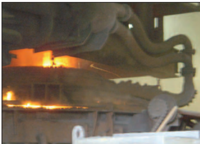
The process starts with melting scrap steel in an electric furnace. When they do this, Arkansas Steel becomes the largest power user in the entire county.
