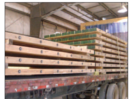
Then, steel dowl rods are inserted and bolted in place before loading onto trucks for shipment. ▶
