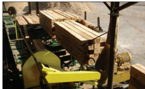
At this mill, they cut for ties first, then re-saw the remaining material. Many people might think it can't be done this way, but this is a very efficient operation, and they do it that way every time.
